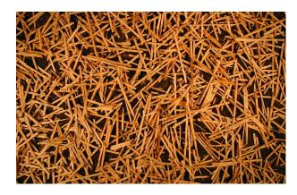
Figure 1. Manufactured wood strand erosion control mulch applied at 70% soil cover.
