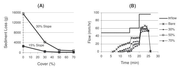
Figure 2: Sediment loss (A) and runoff hydrograph (B) for varying cover amounts of wood strands.
