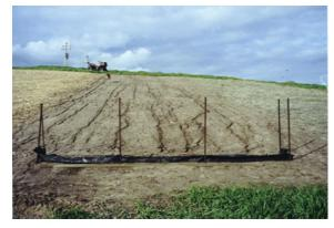
**Figure 7:** Ernst site on January 3, 2005 with wood-strand plot on the left, bare soil in the center, and barley straw plot on the right. As of this date, neither of the treated plots showed any signs of rill erosion while the bare soil plot is heavily eroded.
