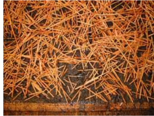
Figure 2. A “look alike” 2002 prototype blend of engineered wood-strand material at 70% soil cover.
