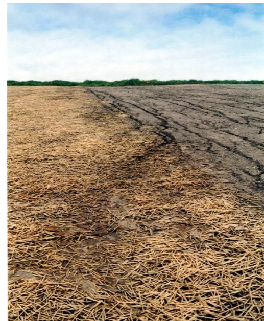
Figures 6. Wood-strand erosion control material on test plots applied at 70% soil cover.
