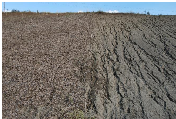
Figures 7. Hand application of wood-strand mulch at 70% soil cover on a 51% slope in Colorado in a CDOT test and follow-up two months later.
